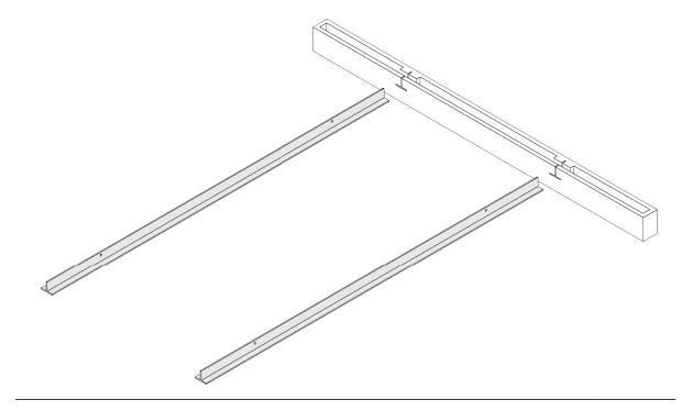
2) Insert the aluminum T-track into the End Cap Beam as shown below:
