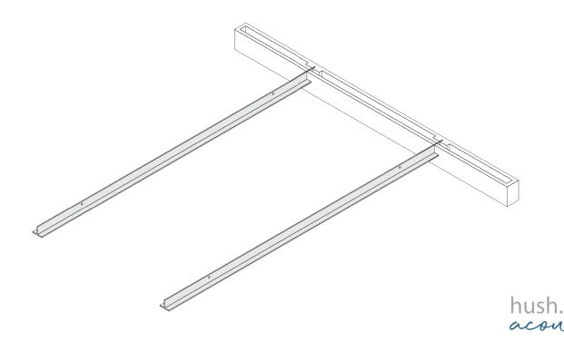
3) Now slide on the intermediate Beams (in numerical order if noted on the Beams ), spacing the Beams using spacing tool provided.
