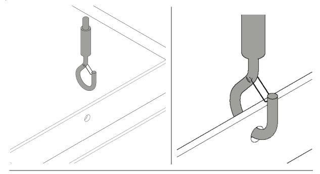
6) When all Clevis-Hooks have been installed, your Linear Beam is now complete and ready to be suspended from the ceiling. (Please refer to the 'Ceiling Hardware Install Guide' for the final steps).
