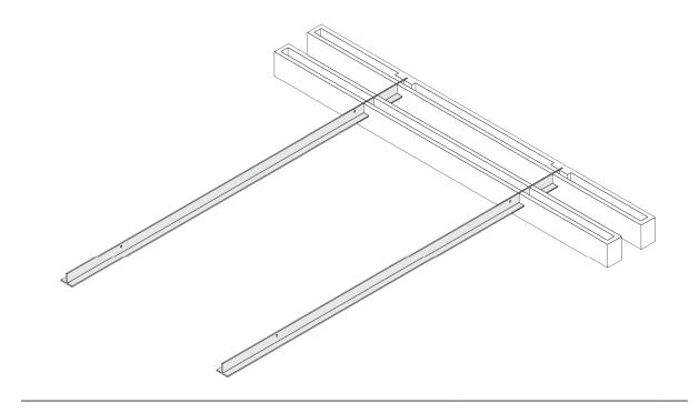
4) Add remaining Beams, ending with a Beam End Cap.
